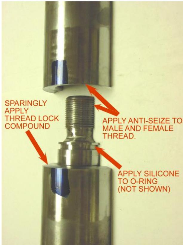
10. Apply anti-seize generously to both the male & female threads. Do not apply anti-seize to o-ring. Apply an o-ring safe silicone to the o-rings of the plunger and cylinder. Use a generous amount of silicone on o-rings, o-ring grooves, and immediate areas.
