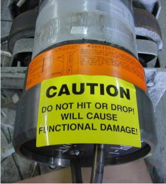
Make sure that all shipping packing is in place at the bottom of the jack sections. If the shipping material is missing or looks like it was damaged check the plunger ends for any type of damage. Any damage (ding or scratch) may result in poor sealing surface or bad parts.
