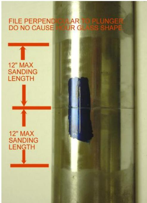
**18.** With rags still in place clean excess Loctite from the joint. If there is no lip experienced over the joint (fingernail should not catch on plunger joint), sanding is not necessary. Take an emery cloth or scotch-brite pad and blend in the area 6 to 12 inches above and below the joint as required.
