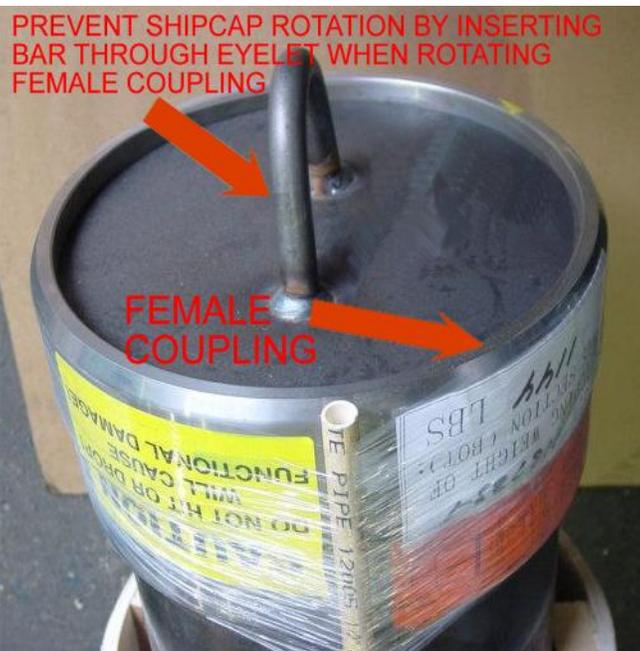
2. After the bottom section is securely mounted, remove female coupling with spanner wrench or strap wrench to expose plunger for installation of the next jack section. The female coupling is removed in a counter clockwise rotation. When removing the female coupling secure the eyebolt with a bar. This will prevent the eyebolt from turning with the female coupling. **NOTE:** *Do not unscrew top shipcap at eyebolt because it may jamb shipcap, damage plunger or plunger coupling.*
