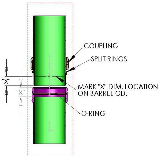
**23.** Check the split rings installed in step #8. They should be installed between the coupling and the shoulder welded to the cylinder. Push down on the coupling until the rings bottom out on the shoulder.
