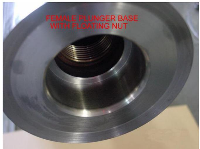
7. Remove bottom protective coating off the intermediate section. (**Note: Split rings are stored under the mesh netting beneath the protective coating. Use caution when removing coating to prevent split rings from dropping into the lower cylinder barrel\***) Clean plunger area of any foreign substance with some type of solvent. Inspect plunger for dings, nicks, or scrapes. If there are any kind of blemishes please contact D.L. Martin at the number printed on the sticker on the jack assembly.
